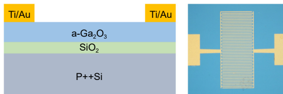
图 1 a- Ga_2O_3 MSM 型日盲紫外探测器结构示意图 (左) 及其显微镜下实物图 (右) Fig. 1 The schematic diagram of the a- Ga_2O_3 MSM SBPD (left) and its microscopic image (right)
