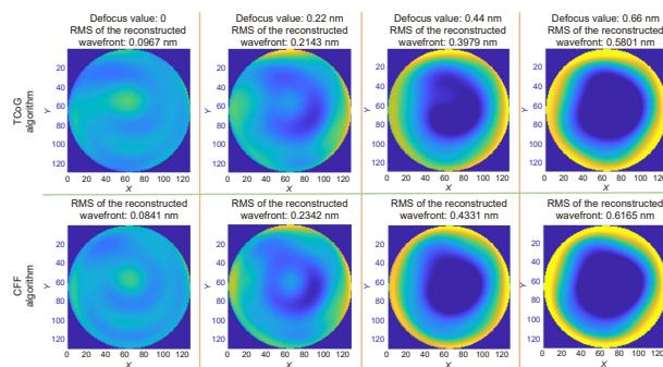
The average reconstructed wavefront using the CFF and the TCoG algorithm. Defocus values are
