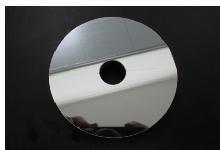
图 7 用于抗辐照性能测试的 \Phi 100 mm 拼接式碳化硅反射镜镀膜后照片 Fig. 7 Photo of \Phi 100 mm brazed mirror after coating for anti-irradiation performance test
