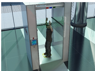
Three-dimensional terahertz imaging with MIMO-SAR
