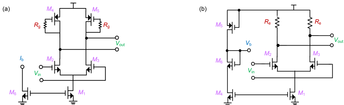
Fig. 7 The large bandwidth amplifier (a) and output buffer schematic (b)
