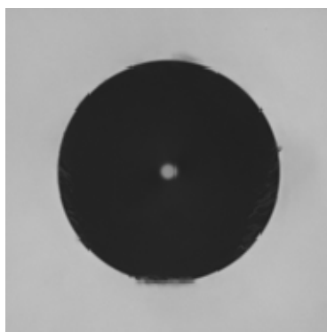
Fiber end face image under improper conditions
