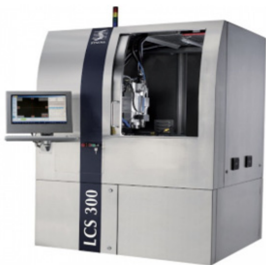
图5 Synova公司LCS300微水导激光加工机床 [37] . Fig. 5 The Synova's LCS300 laser-microjet machine [37] .
