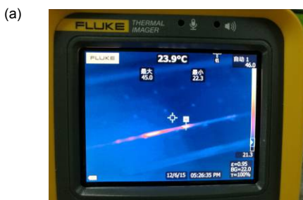
Fig. 9 (a) Temperature of CLS when 209.4 W pump power goes through. (b) Residual pump power output from the CLS vs. input pump power 209.4 W.
