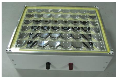
图12 基于非球面透镜的高倍聚光型光伏模组样品 Fig. 12 The high concentrated photovoltaic module sample based on aspheric lens
