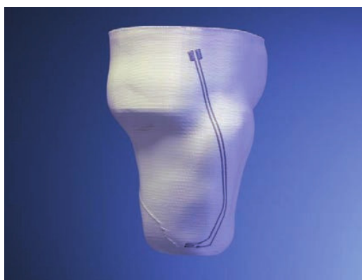
Fig. 12 | Leg prosthesis part produced by FDM and Aerosol Jet printing 31 .
