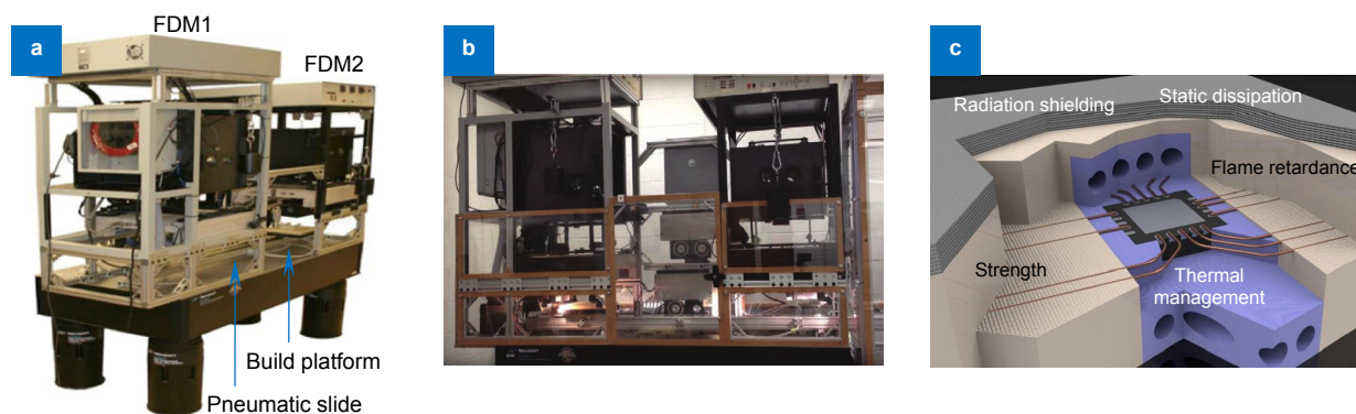
Fig. 1 | (a, b) Photograph of the multi 3D system. (c) Schematic of a fabrication example 9,14
